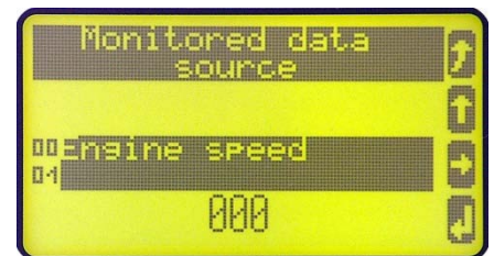
Figure 3-13: Monitoring - flexible limits - data source selection
