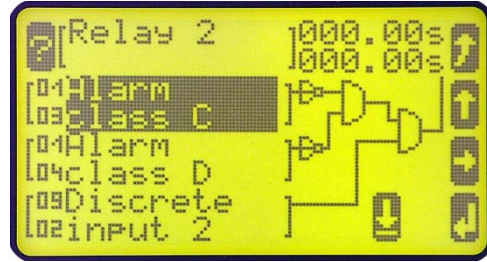
Figure 3-34: LogicsManager - display on LCD screen
