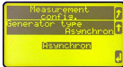
Figure 3-2: Configure measurement - generator type selection
