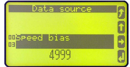
Figure 3-18: Monitoring - analog outputs - data source selection
