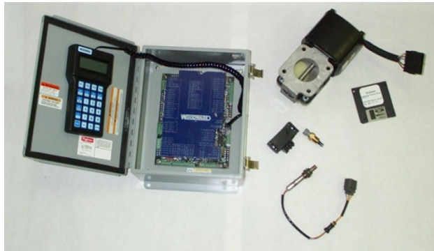
Figure 2-1. System Components with UEGO Sensor
