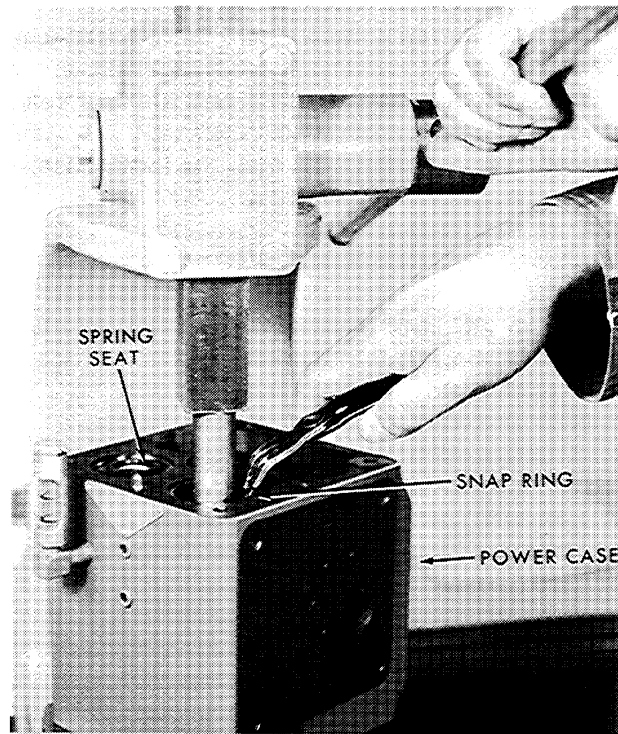
Figure 4-1. Removing Accumulator Retaining Ring
